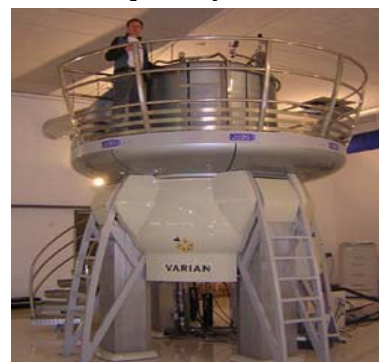
Figure 1. 900MHz, 21.2 T NMR Magnet at HWB-NMR, Birmingham, UK being loaded with a sample.
